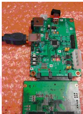
Bridge board connect to device ↑
